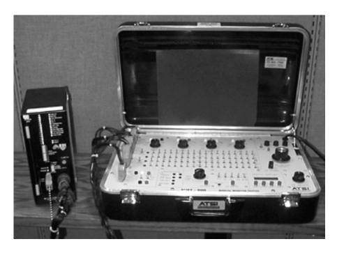
These capabilities are particularly important to signal shops that repair their own monitors. Detailed information on the equipment fault is often required to efficiently track down the failed electronic components. After repairs are effected, the MMT-900 allows verification of a single function of the monitor, before submitting the monitor to an automated test routine.
