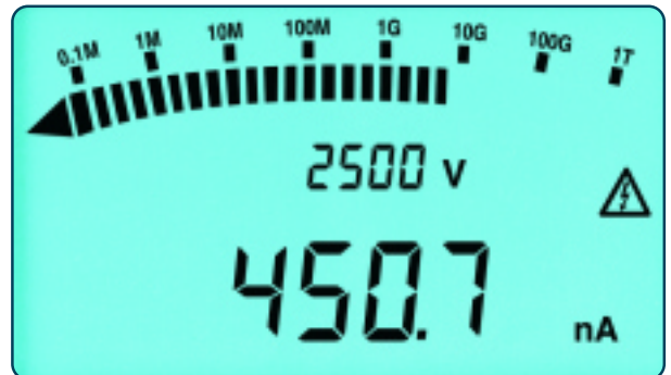
Leakage Current Measurement from 1pA to 3000μA displayed during the test
