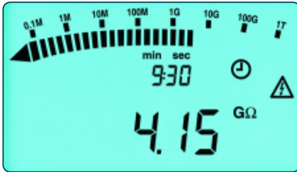
Insulation Resistance Measurement displayed throughout the test
