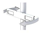
Rotate the lightbar towards the incoming vehicle lane, independent of the wire hole location.
