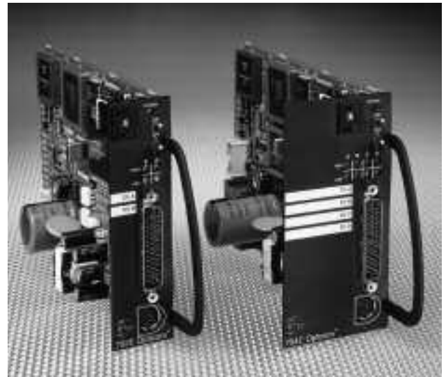
Opticom™ Model 752E Phase Selector (left) and Opticom™ Model 754E Phase Selector (right)
