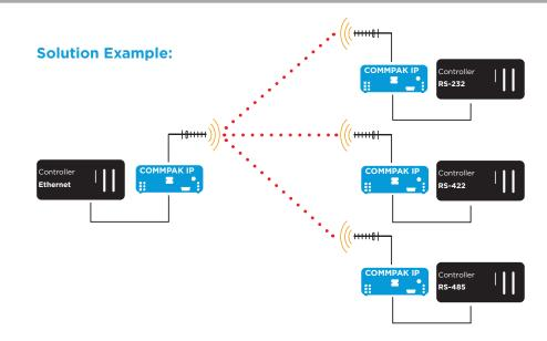
\*\*All interfaces are interchangeable within network and can operate as master, repeater or remote
